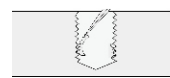
Step 4: Using a scriber remove the remnants of the broken tap flutes.
